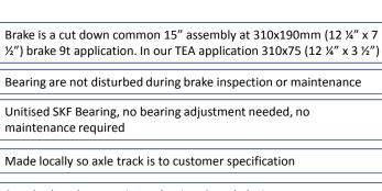
Standard stud pattern is Landcruiser 6 stud, design can accommodate various stud patterns up to a 160mm PCD
